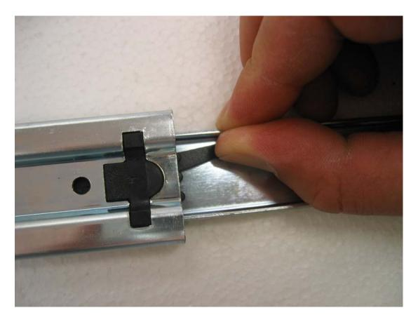
7. Now holding flipped lever with one hand, hold the larger piece with your other hand and pull them apart as shown in the following diagrams.
