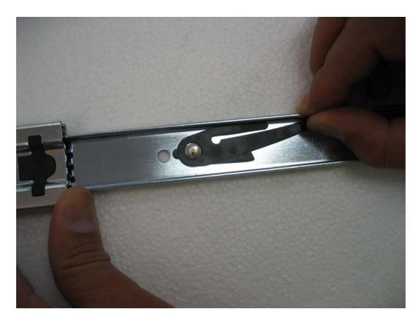
8. The end piece with the lever should slide out and become a separate piece as shown below.
